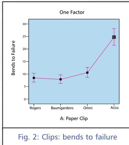
Fig. 2: Clips: bends to failure
