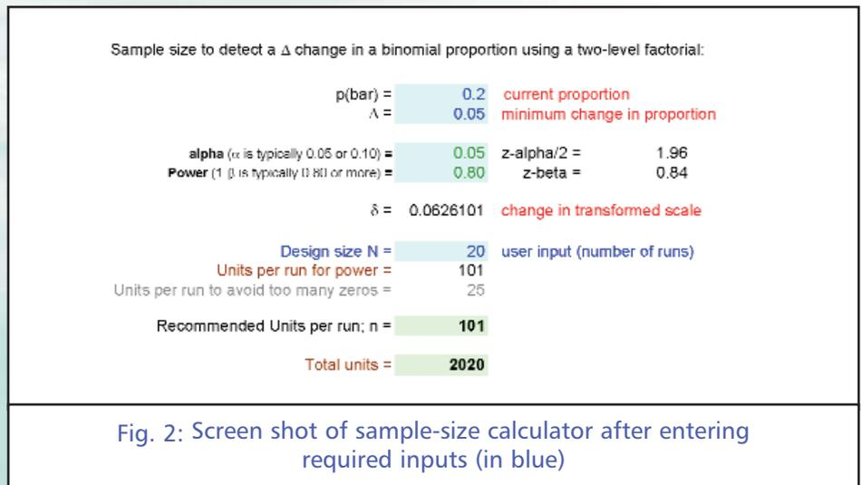
Fig. 2: Screen shot of sample-size calculator after entering required inputs (in blue)
