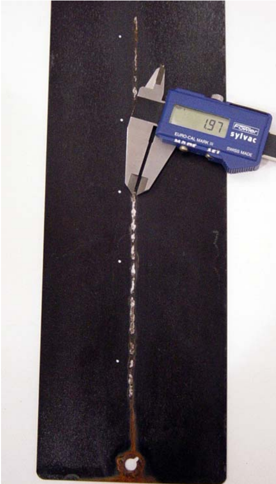
Figure 1: Panel shown after exposure to 504-hr NSS testing.
