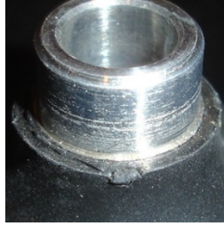
Figure 1: Problematic rubber-to-metal bonding (after destructive peel-back)
